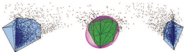
Fig. 6. Monitoring a quadratic function. The set C is the pink ellipsoid, the safe-zones are polyhedra with 12 vertices each (in pale blue), and their Minkowski average is in green.
