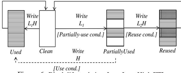
Figure 6: Block life cycle in a Low-Low-High FTL.
